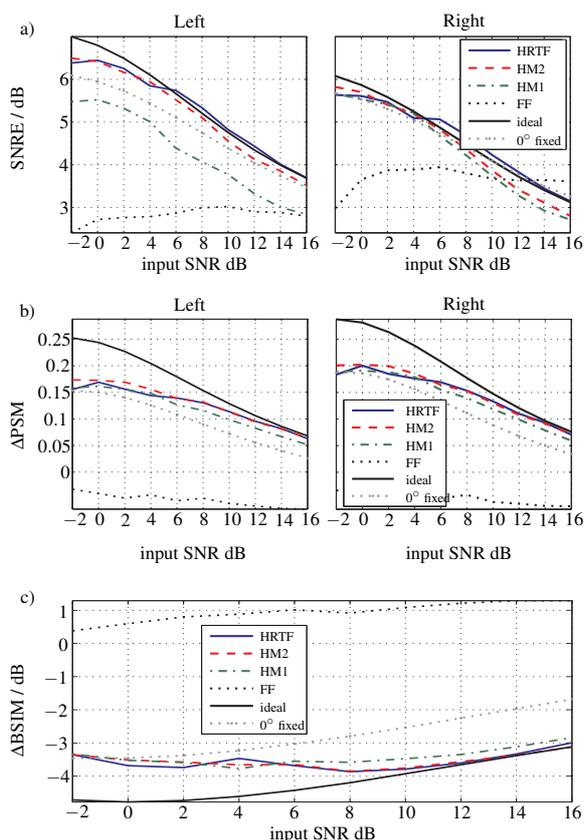
**Figure 6:** Performance evaluation with the objective measures SNRE,  $\Delta$ PSM and  $\Delta$ BSIM for a speech signal in a reverberant office environment ( $\tau_{60} = 300$  ms) mixed with babble noise at different input SNR's and processed by the SRP-PHAT-steered binaural noise reduction scheme.
