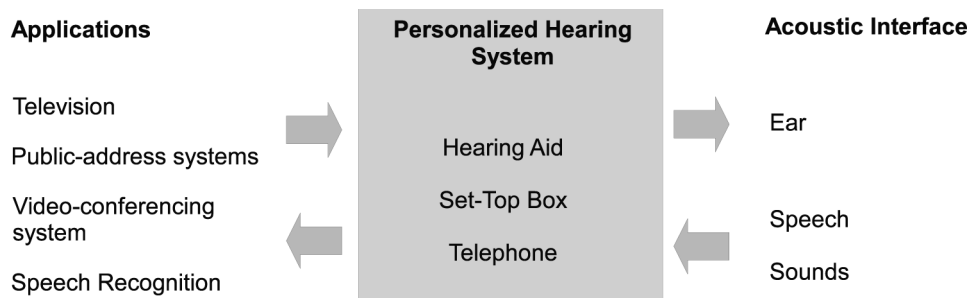
Figure 9. Schematic usage of personalized hearing systems in acoustic human-machine interaction. Applications transmit and receive acoustic information, which is processed in the personalized hearing system for interaction with the user
